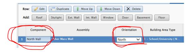
Then input the Gross Area of the first wall (assuming a solid wall – no openings), the U-factor, and the Heat Capacity.
