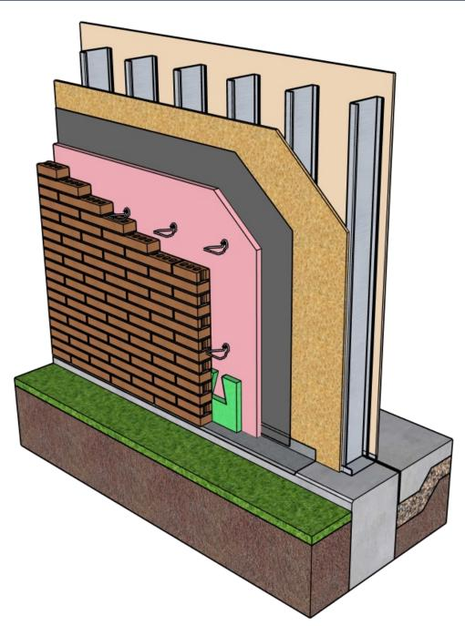
Brick Veneer Over Stud Framing as a Mass Wall: Energy Code Compliance **WITHOUT** Stud Cavity Insulation
